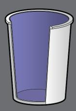
When it comes to maintaining drink temperatures, it's hard to beat a vacuum insulated cup. These cups have the same construction as double walled cups, but the air is removed between the two walls to create a vacuum. A vacuum reduces the rate of temperature change significantly, keeping the outside of the cup cool and preventing messy condensation from cold drinks.
