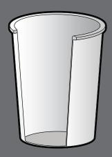
Coffee cups with double wall construction are an economical way to insulate your beverage. The cup is designed to trap air between an internal and external wall. Air has excellent insulation properties and reduces the rate of temperature change. The outside of the cup remains comfortable to hold, and there is no messy condensation from cold drinks.
