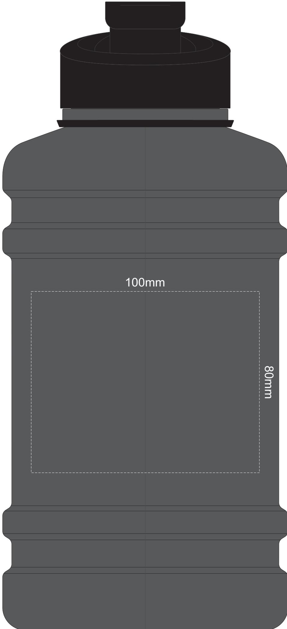
*Block artwork is not recommended due to mold seam.*
